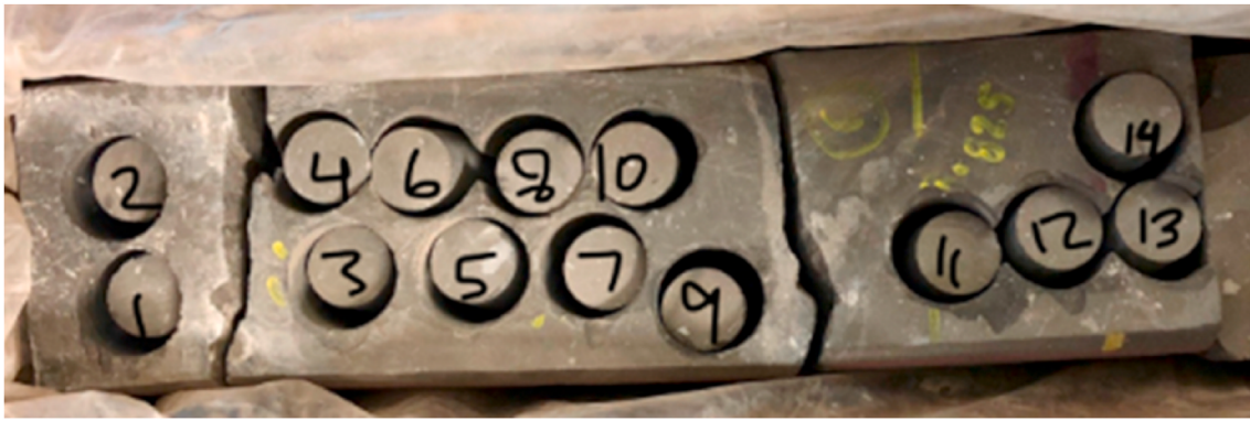
Fig. 2. Core Plugs cut from the Wolfcamp A formation in Martin County.
